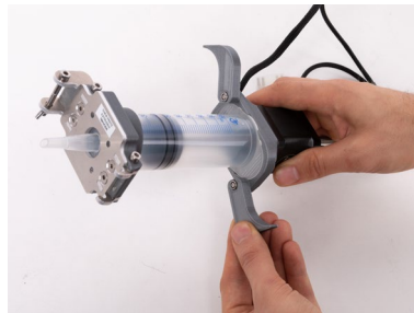
Unlock the syringe blockade.
