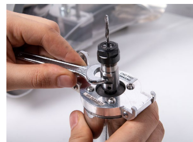
Slide 13-sized end of wrench into shown slot.
