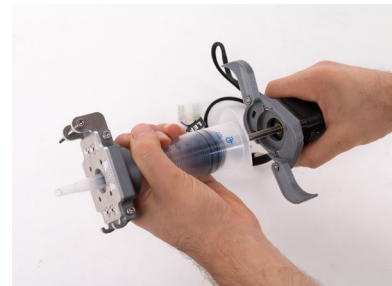
Pull the piston out from the syringe.
