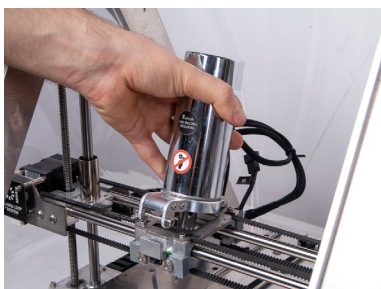
Remove CNC Pro tool-head from your machine.
