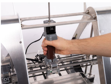
Put the Thick Paste toolhead on the X-cariage mount.
