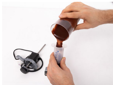
Fill the syringe with the prepared material.
