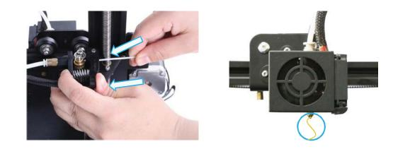
Press and hold the extruder lever then insert 1.75mm filament through the small hole of the extruder. Continue feeding until you see filament come out the nozzle.
