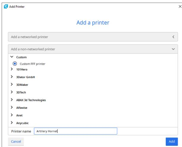
In the **Add a non-networked printer**, scroll down to **Custom** and choose **Custom FFF Printer**, and type in **Artillery Hornet** in **Printer name**. Then click on **Next** button.
