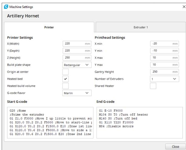
Set **X (Width)**, **Y (Depth)** as **220**, **Z (Height)** as **250**. Make sure **Heated Bed** is checked, then copy and replace the content of **Start G-code.txt** and **End G-code.txt** on the memory card to the respective fields.
