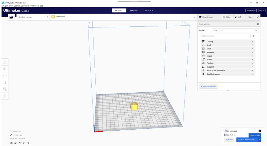
You can click on **Save to Removable Drive** (if the memory card is detected) or **Save to file** button to save the sliced file to the memory card.
