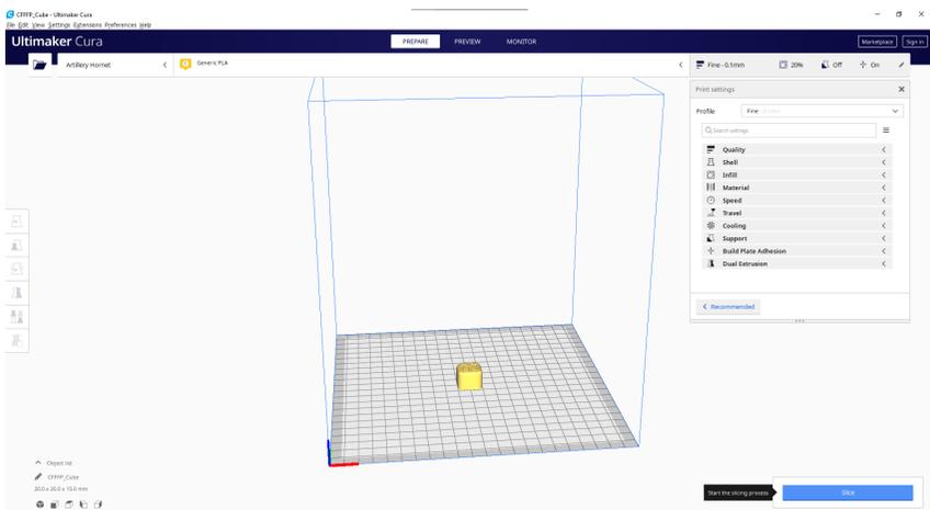
Drag and drop the STL file (or other supported format) to the slicer or load the model file with **File -> Open File(s)...** then click on **Slice** button.
